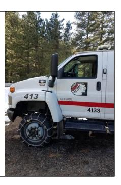
Generally, we chain only the rear axle, for some trucks like 4133 we have front and rear chains. This makes this truck a good option for climbing Nugget hill in snow.
